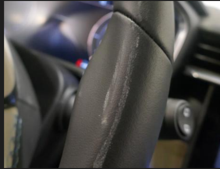
Wear on steering selector and gear shift with respect to the car's age and mileage.
